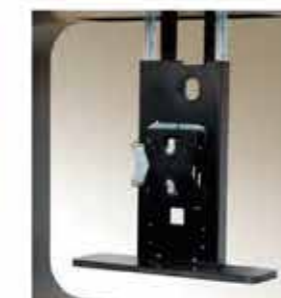
One-motor, belt-driven mechanism for automated sliding
