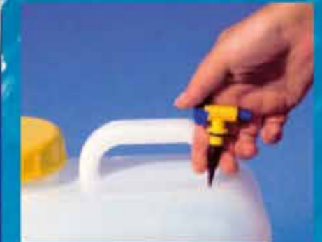
▲ vent valve: Put assembly tip at the side of the O-ring. Press tip through canister wall. Valve gets stuck.
