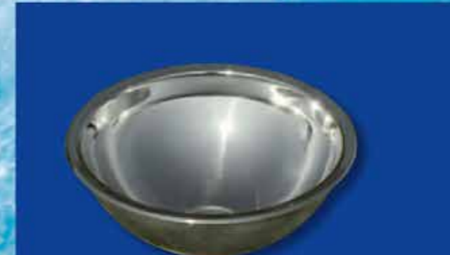
Stainless steel wash-bowl with drain fittings Cutout-diameter: 260 mm Overall-diameter: 295 mm Bowl depth: 120 mm Depth with drain fitting: 150 mm, drain fitting 52 mm, 90° angled for hose 25 mm, with stopper and stainless steel screen. Article code 8730.20.00
